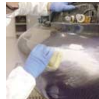
sand repair material
